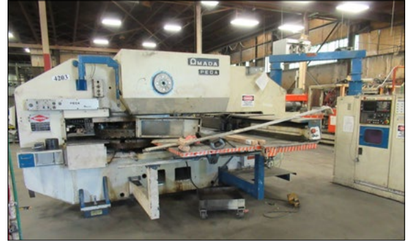
AMADA 30 TON MODEL PEGA 305072 CNC TURRET PUNCH, S/N AA570067, with Fanuc System 6M Control
