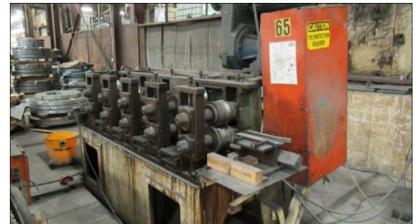
ARDCOR 10 STAND MODEL F10-1-3/4-13 ROLL FORMER, S/N 75-311, 1-3/4" Shaft Diameter, 13" Roll Space, 14" Horizontal Centers, 20 HP Motor 5 STAND ROLLER FORMER, 2" SHAFT DIAMETER, 12" ROLL SPACE, 20 HP MOTOR
