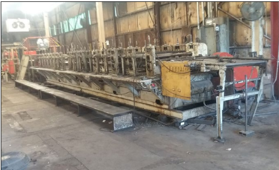
ARDCOR 10 STAND MODEL F10-1-3/4-13 ROLL FORMER, S/N 75-311, 1-3/4" Shaft Diameter, 13" Roll Space, 14" Horizontal Centers, 20 HP Motor 5 STAND ROLLER FORMER, 2" SHAFT DIAMETER, 12" ROLL SPACE, 20 HP MOTOR
