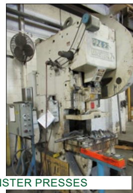
PIRANAH 175 TON MODEL 175-12 PRESS BRAKE
