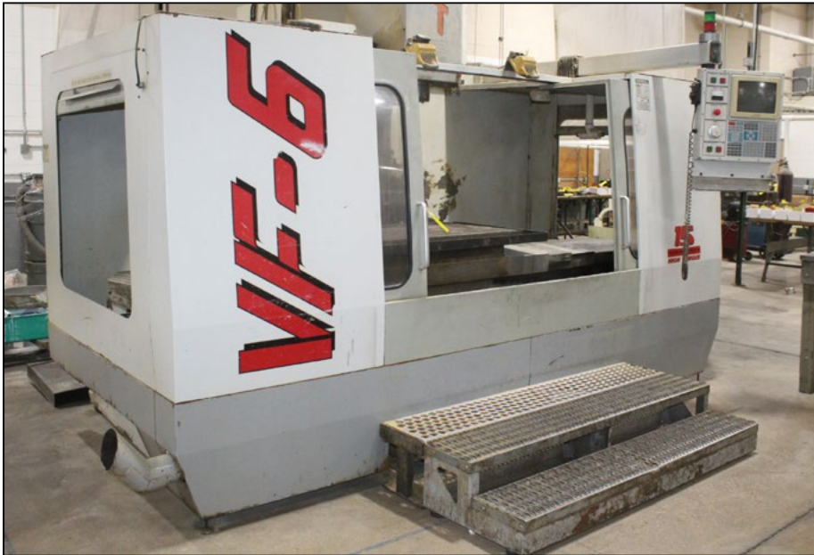
HAAS MODEL VF-6 CNC VERTICAL MACHINING CENTER, S/N 7882, 64" X-Axis Travel, 32" Y-Axis Travel, 30" Z-Axis Travel, 20 Station Automatic Tool Changer, 40 Taper Tooling, 15 HP Spindle Drive, Haas Control
