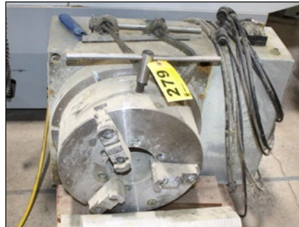
HAAS MODEL HRT-450 4TH AXIS BRUSHLESS ROTARY TABLE WITH 16" 3-JAW CHUCK
